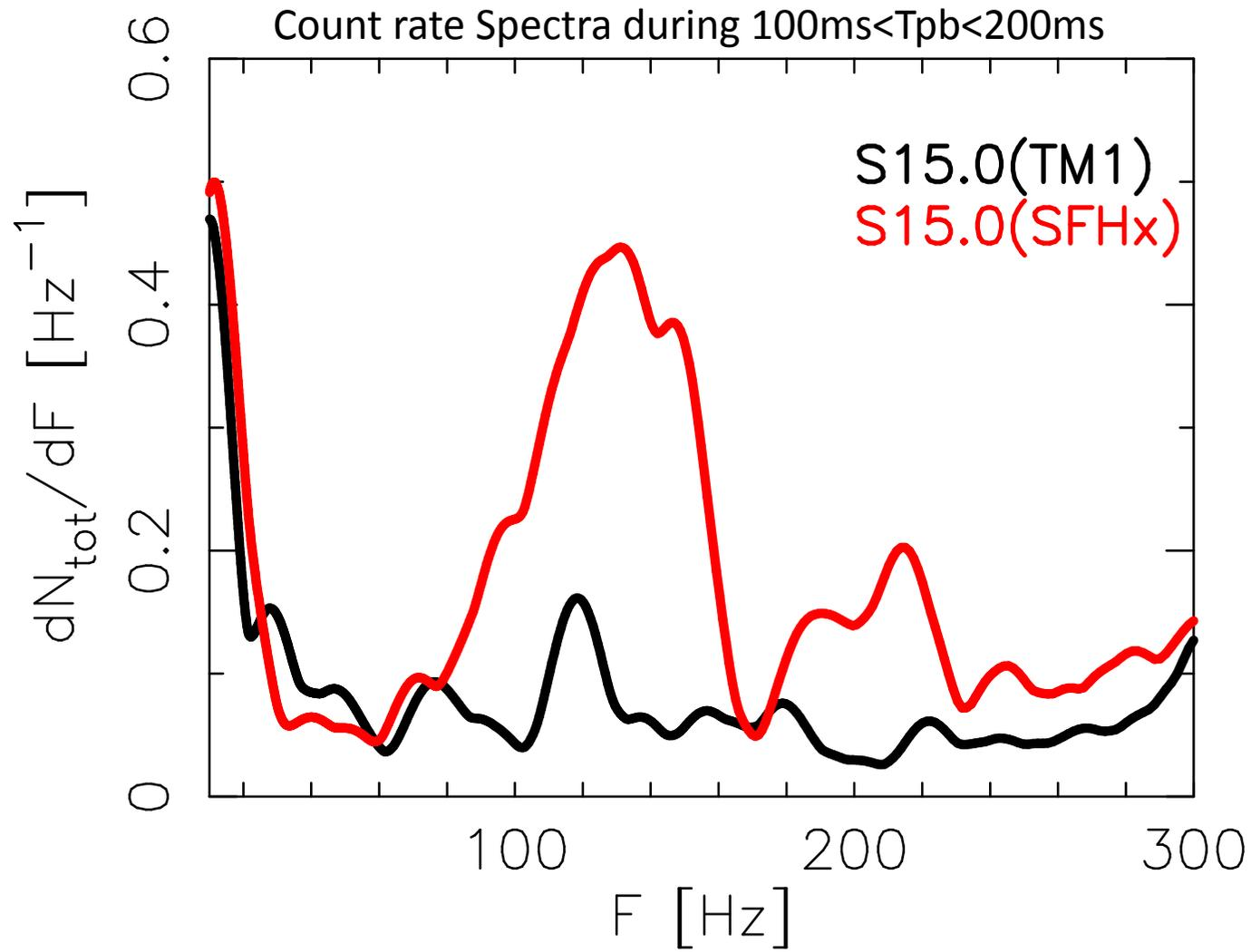
SASI modulation appears clearly at  $F \sim 100\text{Hz}$
